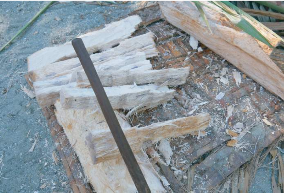
Sago bark is chopped down into smaller pieces before grinding
