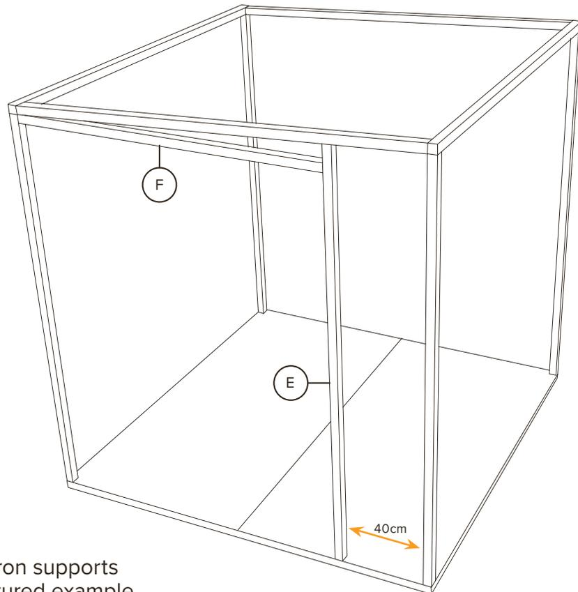
6. Make a door by welding the iron supports in the same structure as the pictured example.
