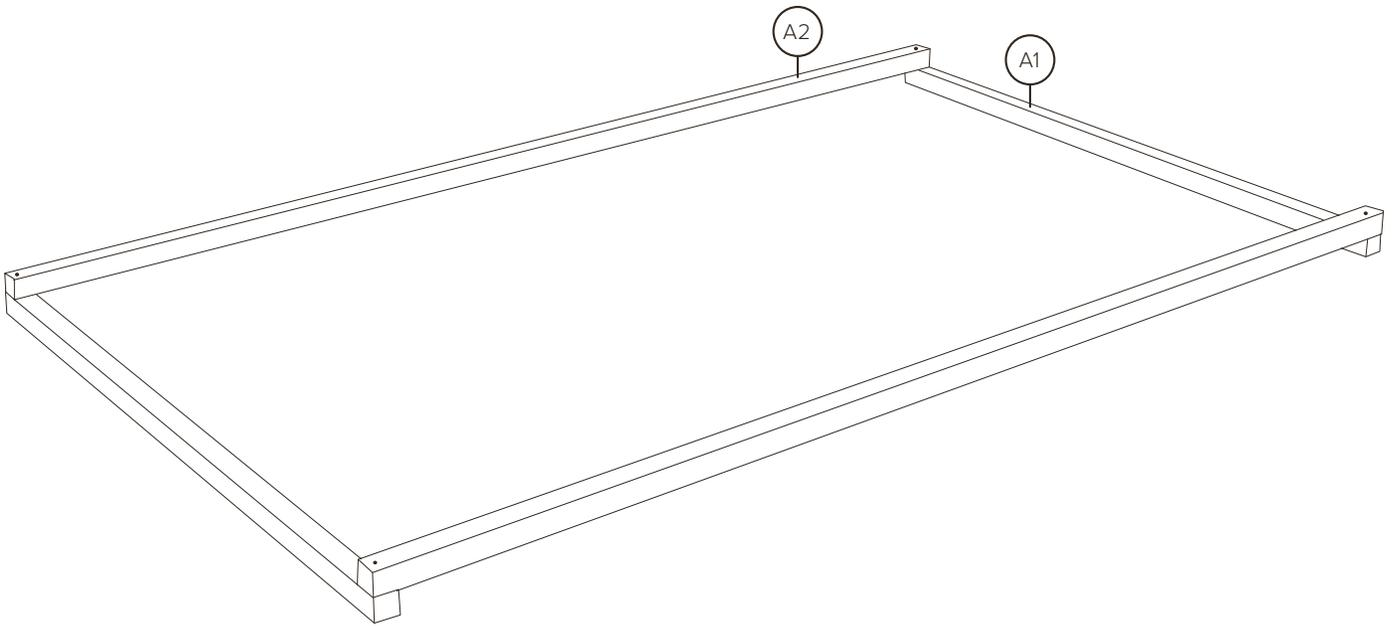
5. Attach the wooden blocks with nails in the same way as the pictured example.
