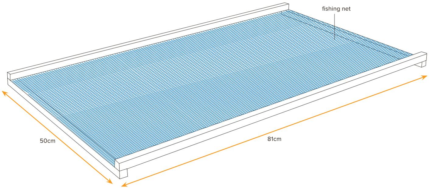
6. Attach the fishing net to the shelf frame with thumb tacks in the same way as the pictured example.
