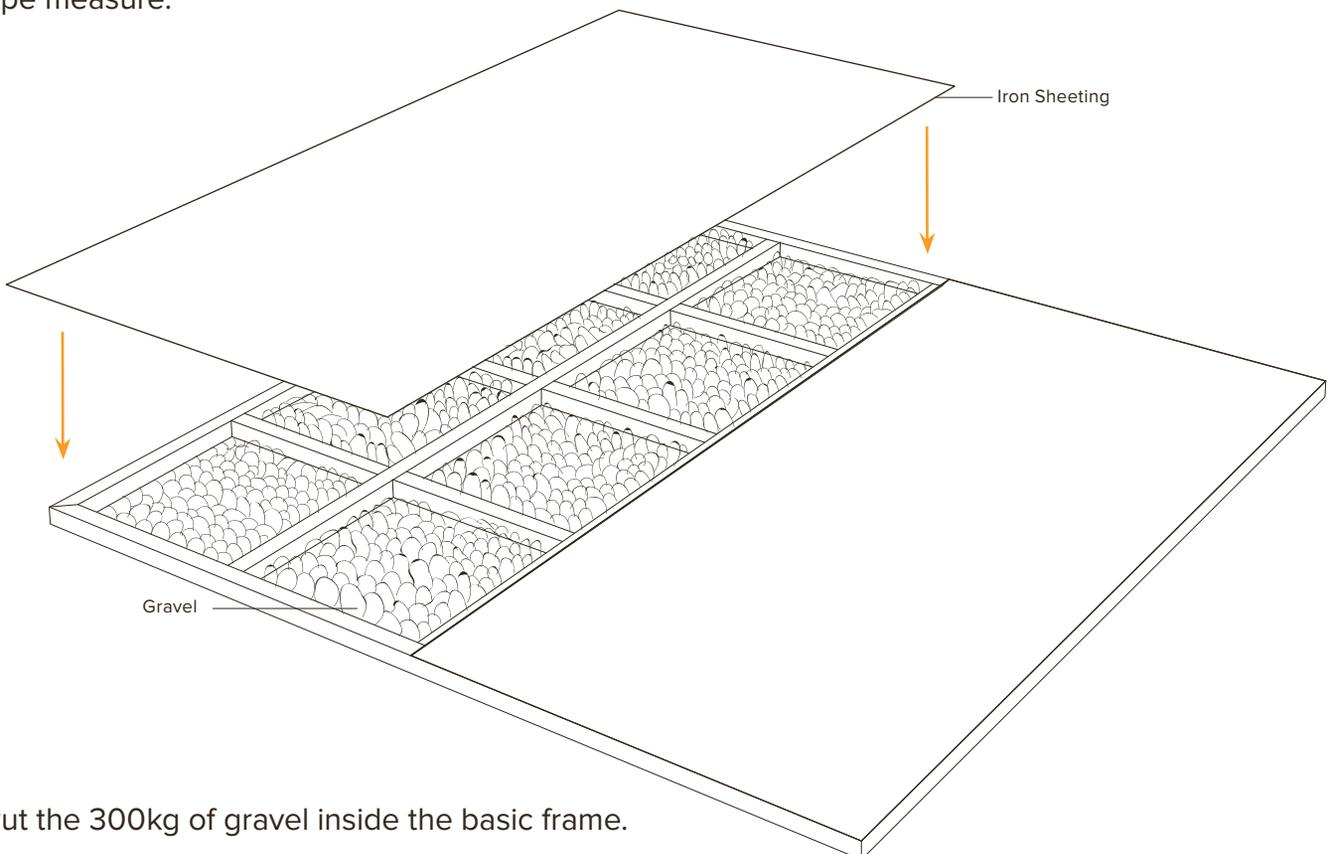
3. Put the 300kg of gravel inside the basic frame.
