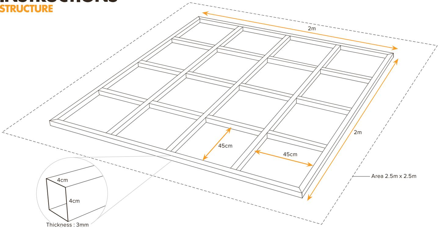
1. Prepare an area of 2.5mx2.5m. Ensure that the area is flat by using a split level and is free from rocks and grass.
