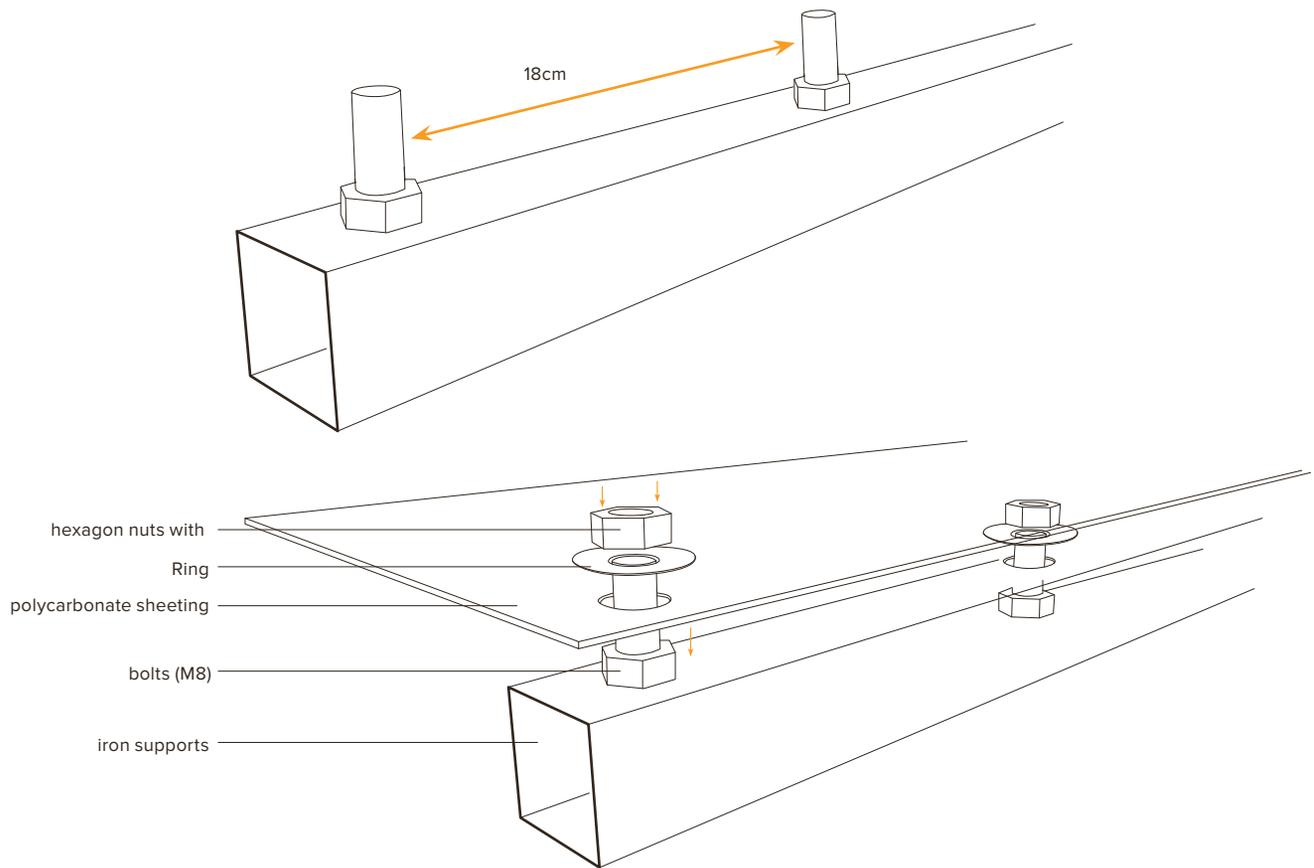
10. Attach the polycarbonate sheeting on to the iron supports, then lock it in place with the hexagon nuts and bolts (M8). The polycarbonate sheeting needs to be securely attached to the frame.
