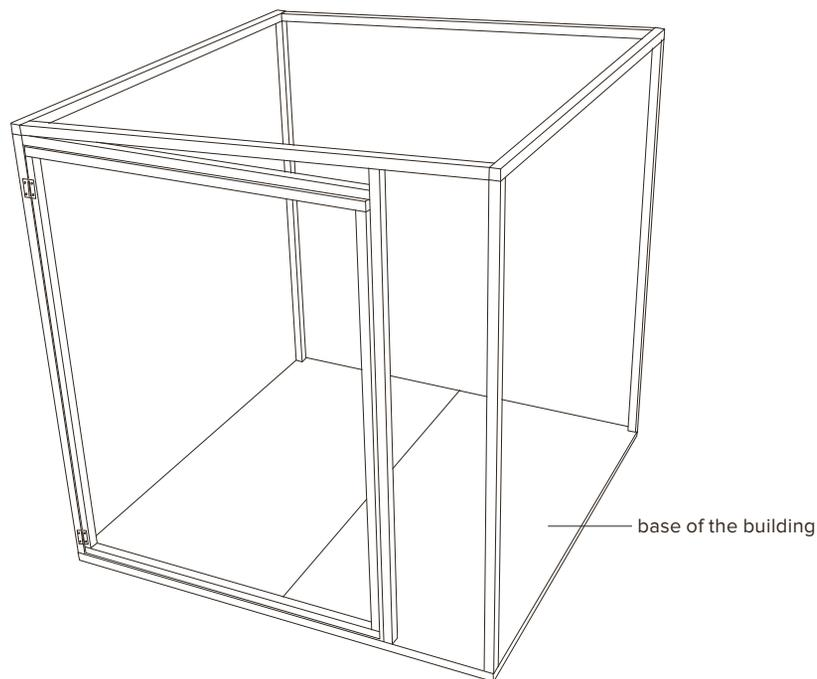
11. After the building is finished, paint the base of the building with black metal paint. While waiting for it to dry, start building the shelves.
