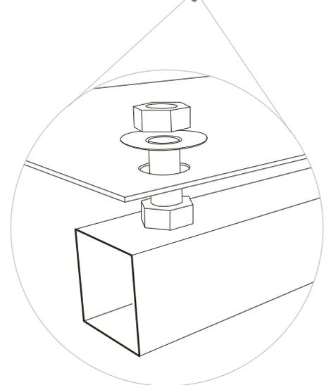
9. Weld bolts onto the surface of the iron supports as pictured in the example, with an 18cm space between each bolt.
