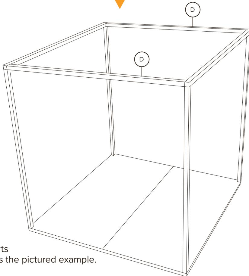
5. Weld the iron supports in the same structure as the pictured example.
