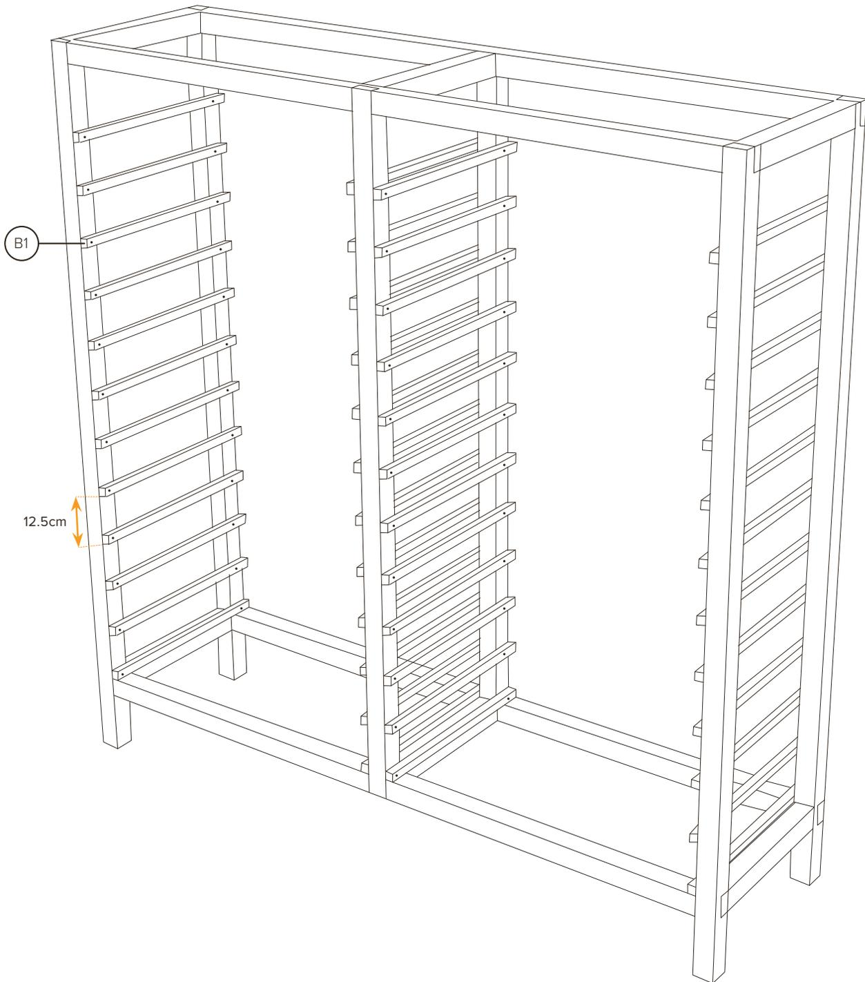
4. Attach the wooden blocks with nails in the same way as the pictured example.
